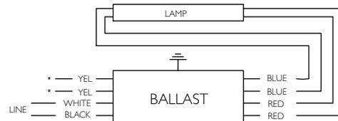
\*FOR SINGLE LAMP OPERATION, INSULATE YELLOW LEADS INDIVIDUALLY FOR 600V
