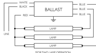
\*FOR TWO LAMP OPERATION, INSULATE UNUSED BLUE LEADS INDIVIDUALLY FOR 600V
