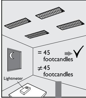
Measure the light level under each MicroLuxSense sensor with no or negligible daylight contribution.
