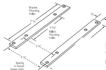
PC-909 Mounting bracket for Fig. 2, 3a & 8 when used with power-door roadway fixtures
