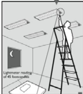
If needed, turn the diaphragm until the required light level is reached (with no or negligible daylight contribution).
