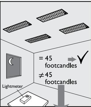
Measure the light level under each LuxSense sensor with no or negligible daylight contribution.
