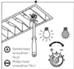
The setpoint of the sensor can be changed manually by using a screwdriver to turn the control ring on the front, which influences the diaphragm. The housing is equipped with an indication of the default setting.
