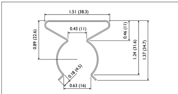
Dimensions of ring LCA8001 inches (mm)
