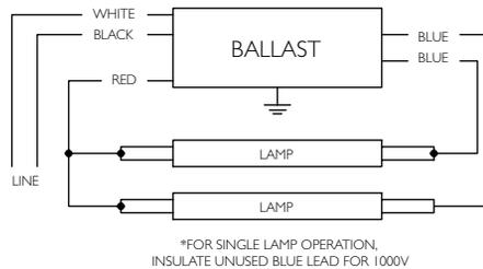
\*FOR SINGLE LAMP OPERATION, INSULATE UNUSED BLUE LEAD FOR 1000V
