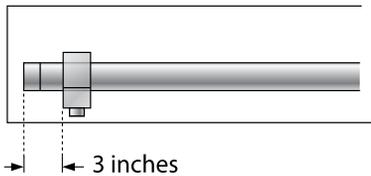
Position LuxSense 3 inches away from the end cap on the (electrical) "cold" side of the lamp. This is the side of the lamp that is connected to the terminals of the ballast that allows for the longest wiring to the lamp.
