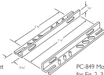
PC-849 Mounting bracket for Fig. 2, 3a, 8, 8a & 10.
