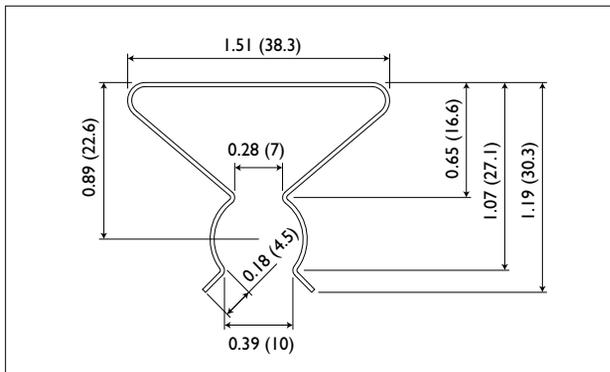
Dimensions of TLD (T8) Clip LCA8003 inches (mm)
