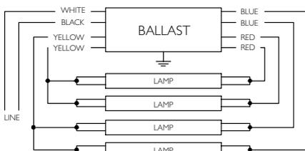
\*FOR THREE LAMP OPERATION, INSULATE UNUSED BLUE LEADS INDIVIDUALLY FOR 600V
