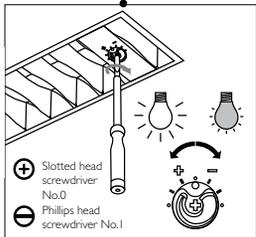
The setpoint of the sensor can be changed manually by using a screwdriver to turn the control ring on the front, which influences the diaphragm. The housing is equipped with an indication of the default setting.
