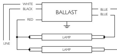
\*FOR SINGLE LAMP OPERATION, INSULATE UNUSED BLUE LEAD FOR 600V
