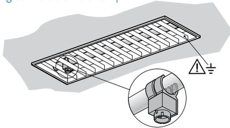
LuxSense mounted with a lamp clip (For use with T5 lamps only).
