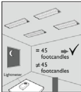
Measure the light level under each ActiLume I-10V sensor with no or negligible daylight contribution.
